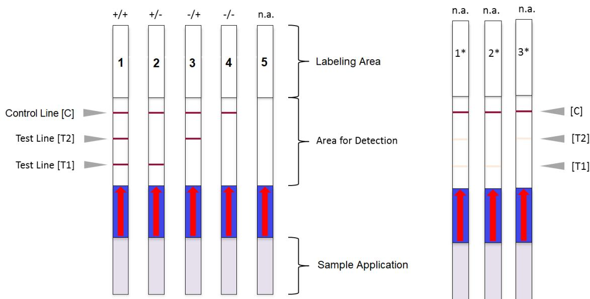
The control line [C] confirms the proper function of the test strip. The test line 1 [T1] is associated with the proper function of the PCR. The test line 2 [T2] is linked with the presence or absence of the *Megasphaera* sp./*Pectinatus* sp. gene.
